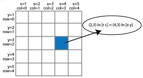
The following MATLAB code converts point coordinates from an [r c] coordinate system to the [x y] coordinate system:
